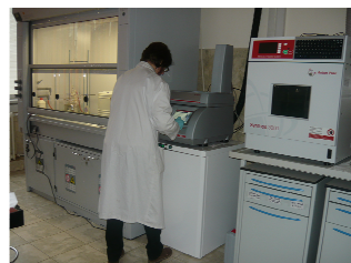
Nisa chimica de laborator & Instalatie de tratare probe in camp microunde
